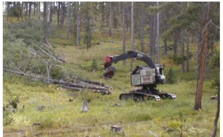
Use of a feller-buncher and directional felling can help minimize soil disturbance in the SMZ.
