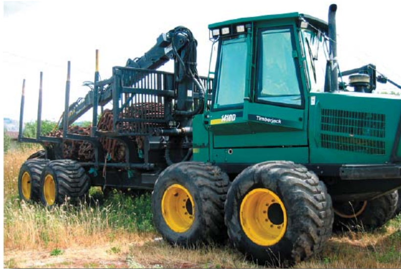
The Forwarder has a log bunk and a crane with a grapple, so the logs are carried out of the woods, not dragged.
